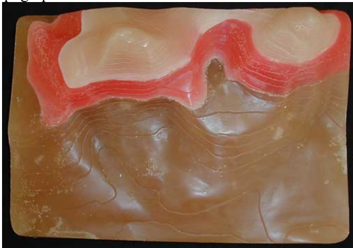
Fig. 2: Top (map) view of wax model showing the constant, uniform outcrop pattern produced by flat-lying strata (top = map view).
