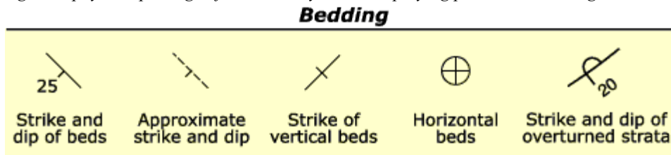
Fig. 2: Symbols used to denote the orientation of tabular sedimentary beds or strata.
